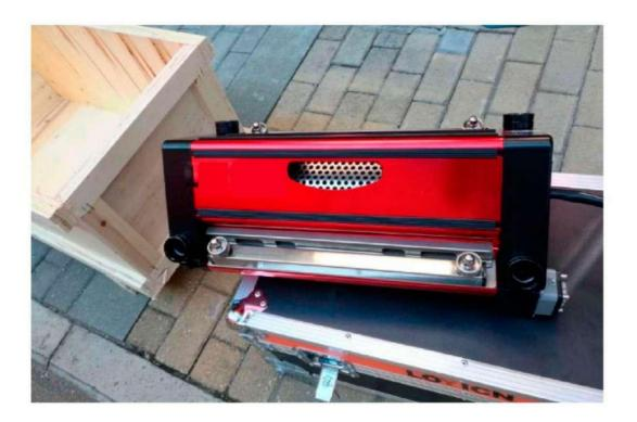
The splice press is an all-in-one solution for splicing thermoplastic conveyor belts (e.g. PVC polyurethane). They were designed to splice right on site. It's an air-cooled design, portable press specifically made for PVC/PU conveyor belts. No external control box, air pump, or water cooling tank are required. Everything is built right in. Make the splicing easier and more efficient, shorter the belt won't run time and increase the production rate.
