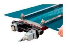
Have two clamp bars, that can set the belts fingers remain tightly meshed and keep in a horizontal line.
